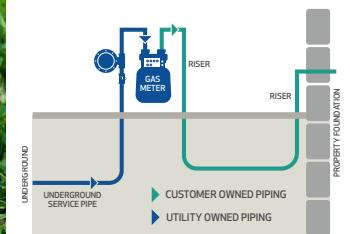
It's important to understand that property owners are responsible for the maintenance and inspection of buried piping from their gas meters to structures like homes, businesses, and other facilities, and aboveground piping from the meter to structures or gas utilization equipment.
